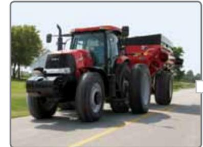
Auto 4WD and Diff lock disengage and engage automatically e.g. on tight corners, when braking and depending on hitch position and forward speed.
