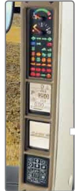
An A-Post instrument cluster with an optional performance monitor tracks important functions and data for convenient at-a-glance monitoring.
