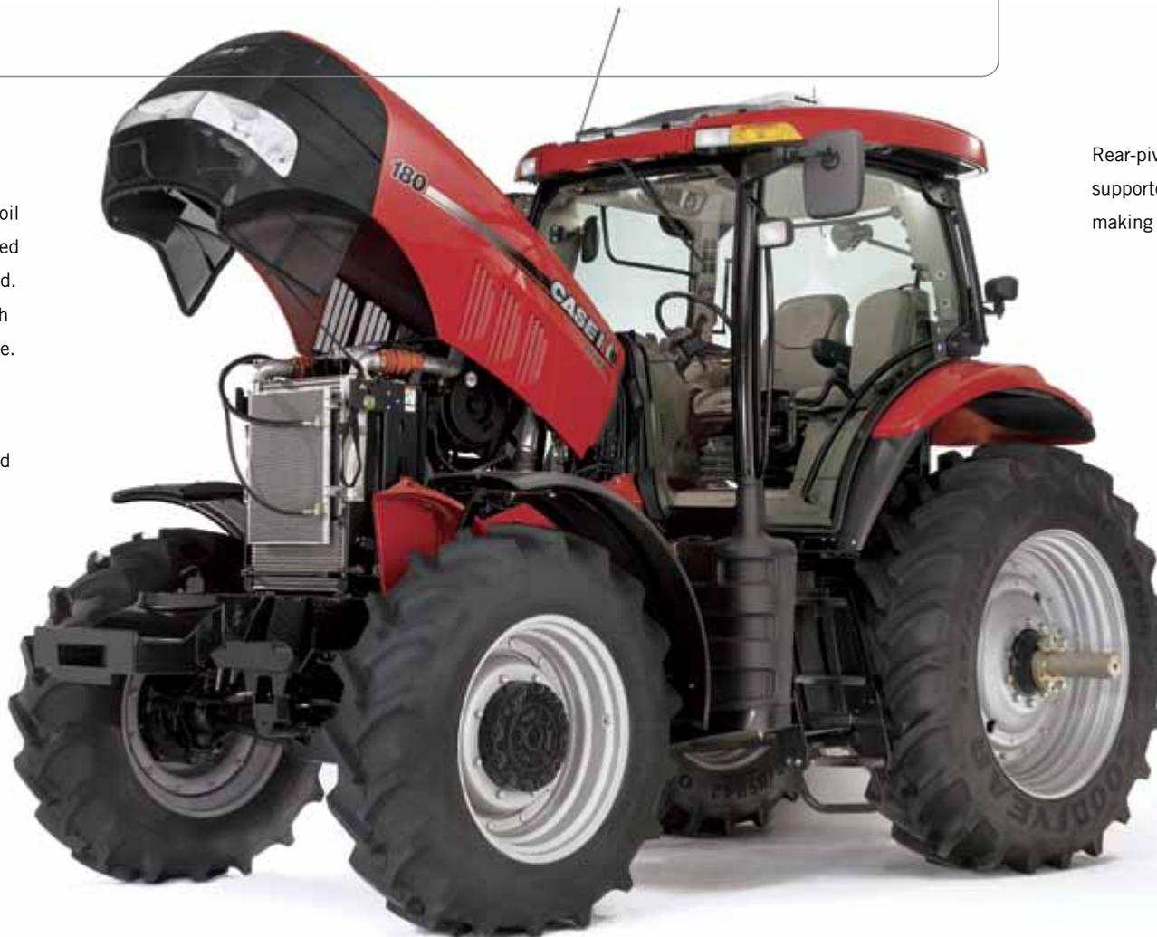
Rear-pivot front-release hood is supported by gas-filled cylinders, making it easy to raise.
