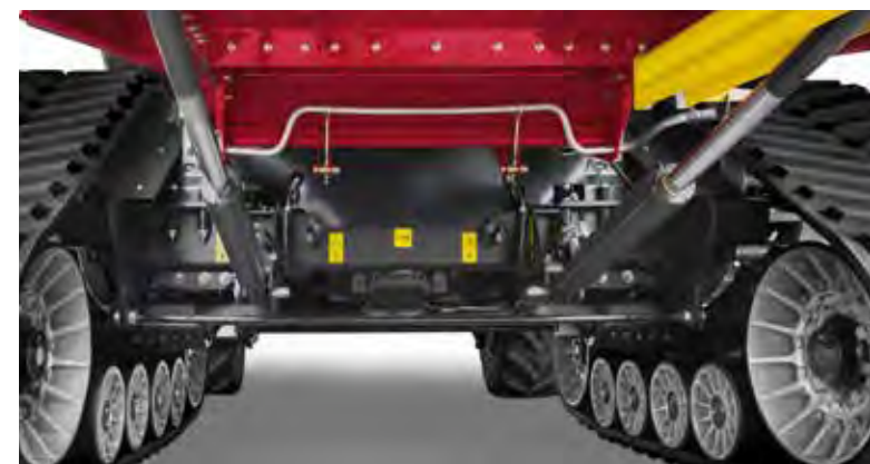
Repositioned lift cylinders for higher lift capacity. Dual lift cylinders for improved header height control
