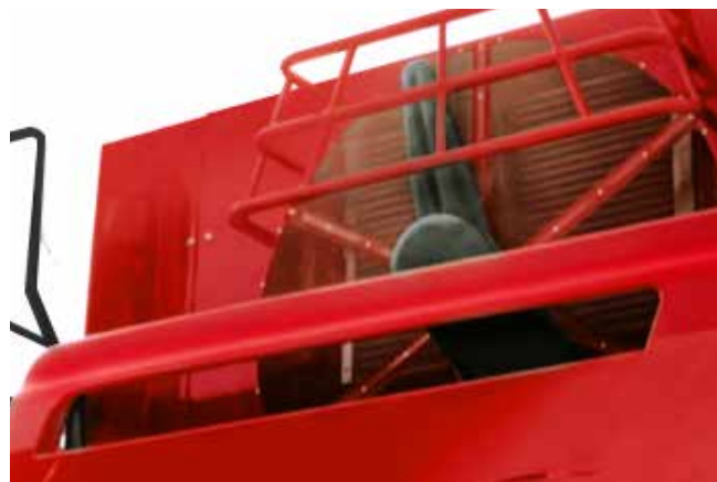
Fixed radiator grille for optimal dust clearing
