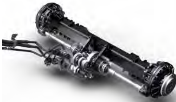
New hydrostatic drive and transmission for increased traction. Oil cooled brakes offer constant braking power
