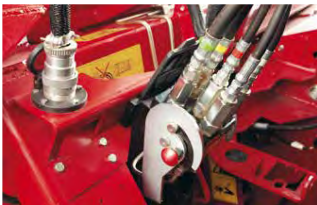
Mount the header in a matter of minutes with the single latch that connects all hydraulic and electric services
