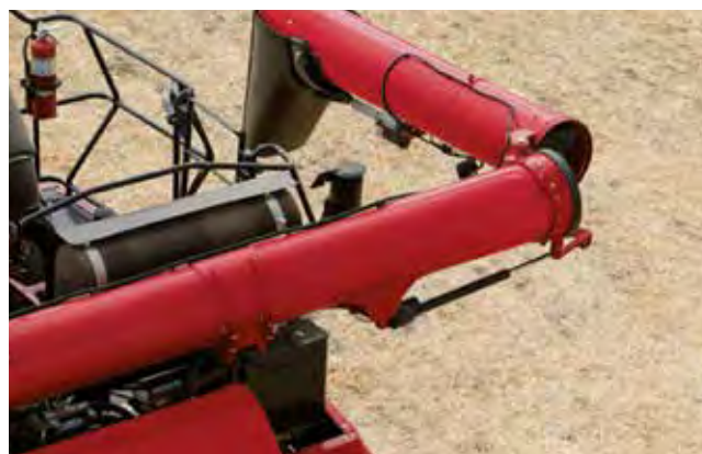
The 8.8 m and 10.4 m unloader augers are available as foldable versions for easier transport on the road and for easier manoeuvring in sheds for storage
