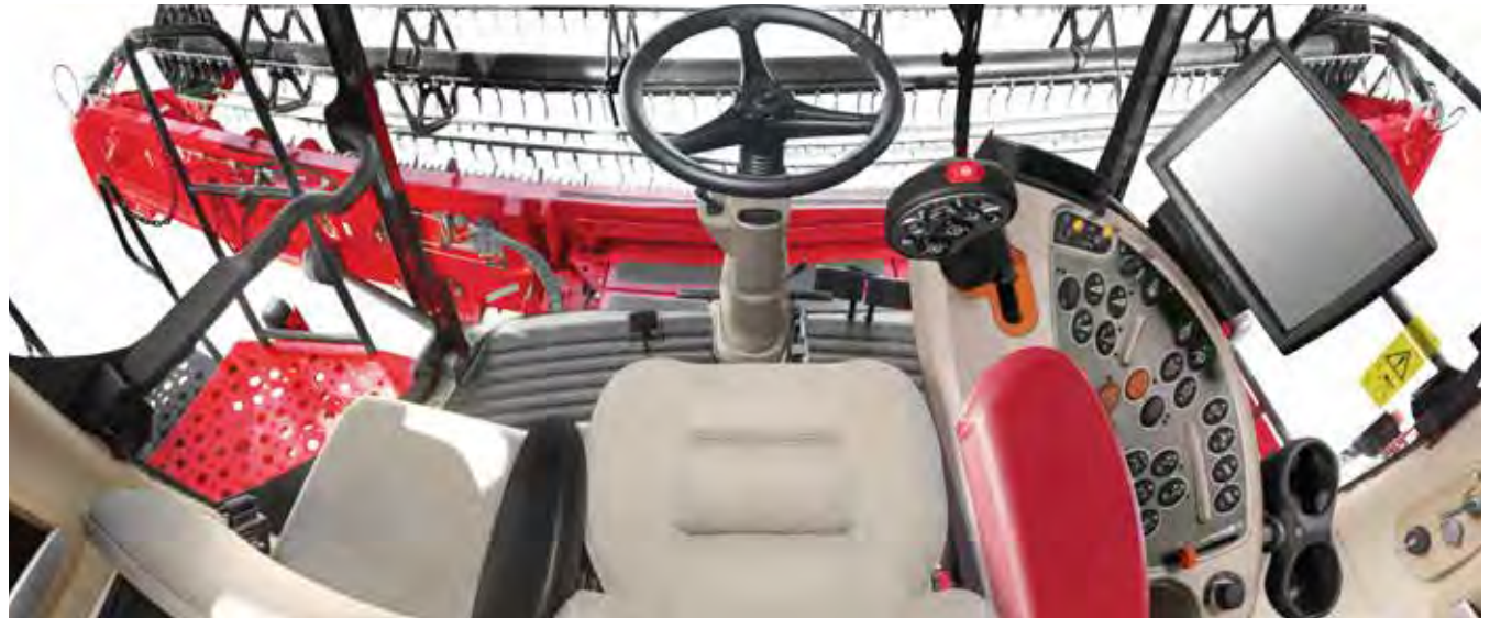
Comfortable cab, full view of the header and ergonomically laid-out control console
