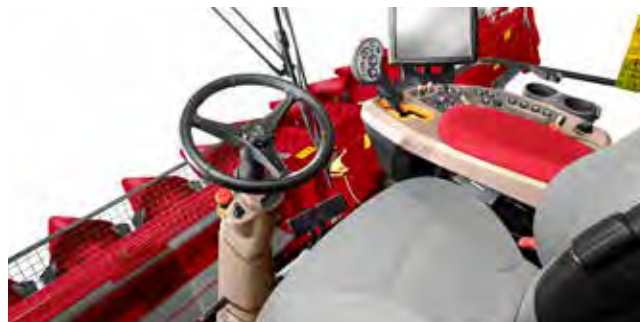
Foldable steering column with new emergency switch and telescopic extendable steering wheel - no obstruction to the view
