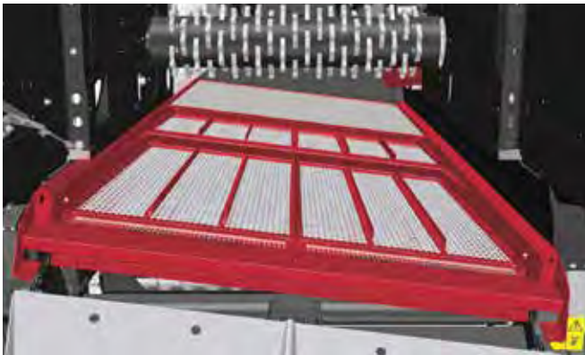
Large self-levelling sieve surface ensures excellent cleaning performance
