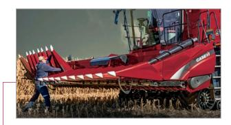
■ The 4400 series narrow spacing is engineered to achieve overall weight reduction and better center of gravity. This is achieved keeping strong transmission via gearboxes (without chains) and Case IH patented design hoods.
