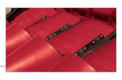
Grain-saving, patented CornLouvers™ direct grain back toward the auger to ensure loose grain makes it into the combine.
