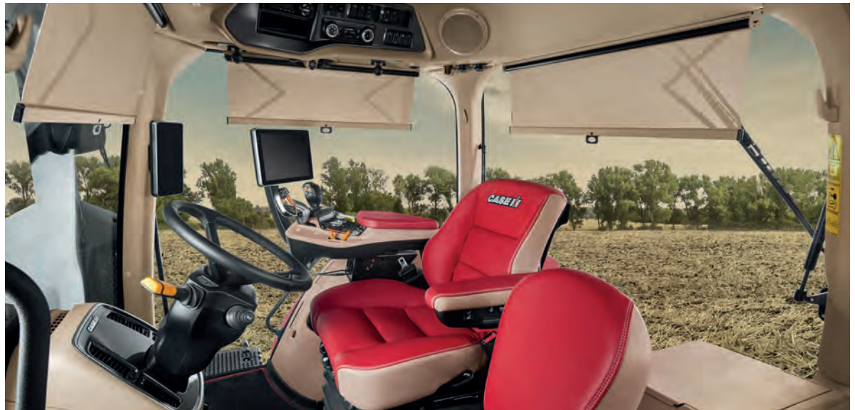
The semi-active, hydraulic cab suspension reliably absorbs jolting and vibrations.
