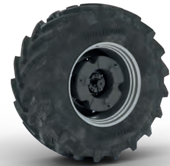
Rear wheels weights are available of up to 2,500kg in total.
