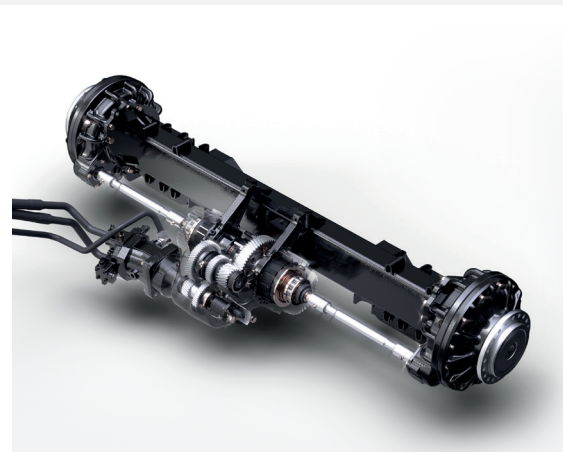
New hydrostatic drive and transmission for greater traction. Oil brakes have consistent braking power.
