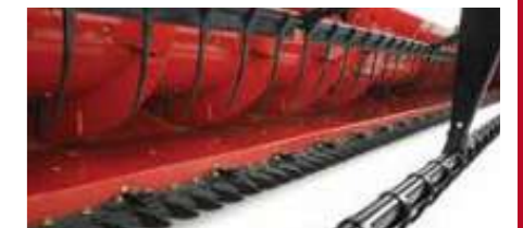
Grain header: endless with a larger diameter, with Full-length retractable fingers
