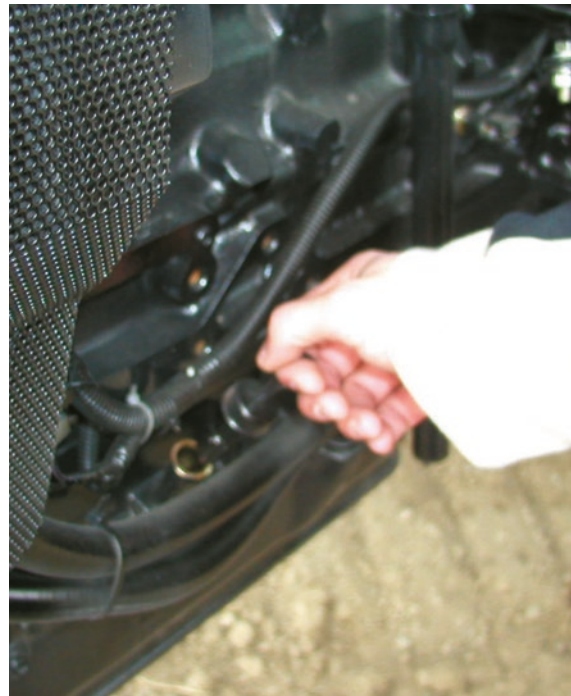
Engine checking oil check without lifting the hood.
