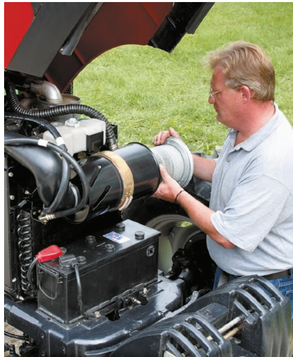
The filter can be removed without tools, making maintenance faster.
