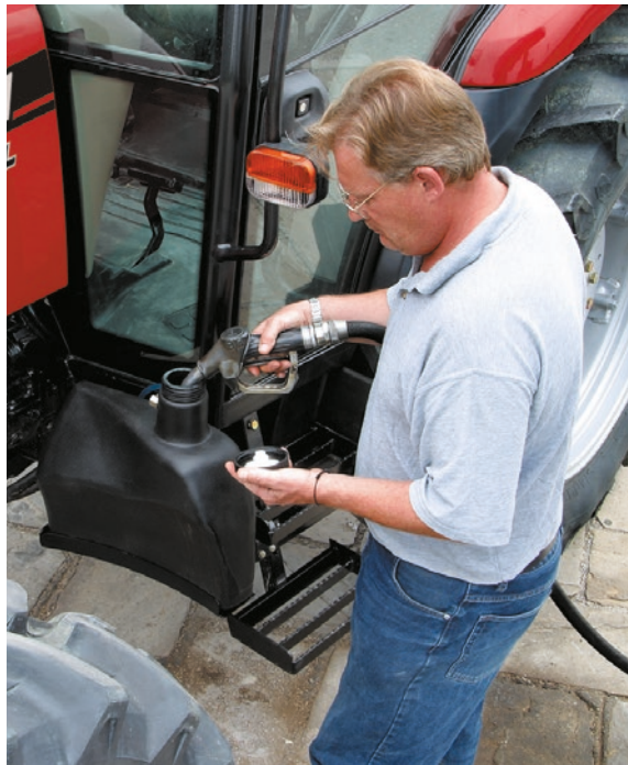
Refueling from the ground with easily accessible filler neck.
