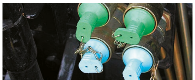
The remote valve auxiliary system offers two rear valves.
