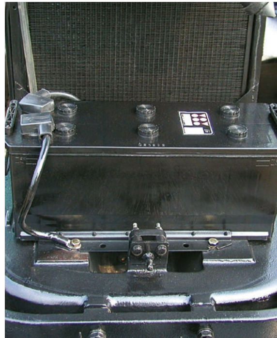
The battery is mounted under the engine hood at the front of the tractor.
