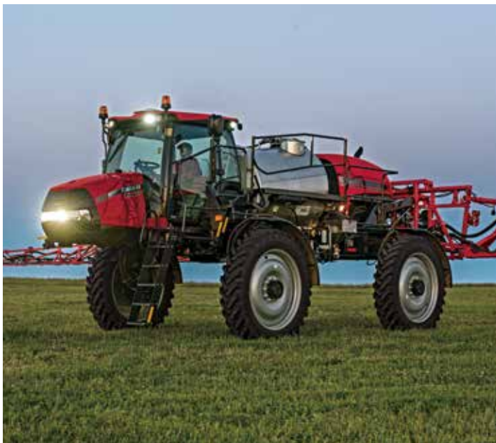
Case IH equipment, like this Patriot 3340 sprayer, is designed to deliver even weight distribution, which means less rutting and soil compaction in wet conditions.
