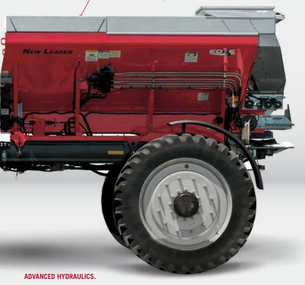
At the heart of the precision dry product applicator is a hydraulic system that supports precise, independent spinner speed and conveyor control. System sensors and alerts, plus automatic chain tensioners greatly extend conveyor life.
