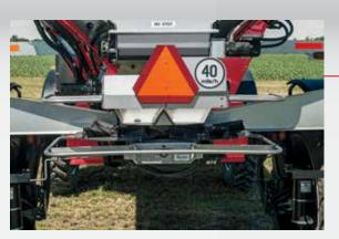
The NL4500T G4 Edge features patented precision spinner technology that allows it to spread product faster, wider — dry fertilizer up to 120 feet and ag lime up to 60 feet — and more consistently.
