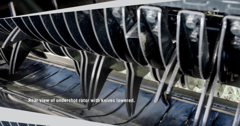
Rear view of undershot rotor with knives lowered.
