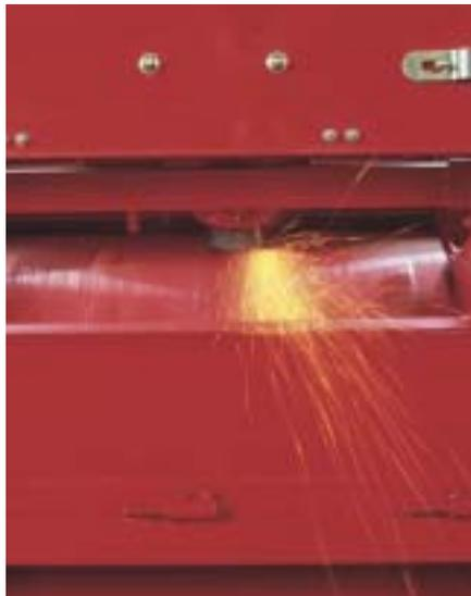
In minutes, you can sharpen knives for uniform cutting and top fuel efficiency. A large, 3-in.-diameter sharpening ratchet-advanced stone passes over the length of the knives for an evenly sharpened cutterhead.
