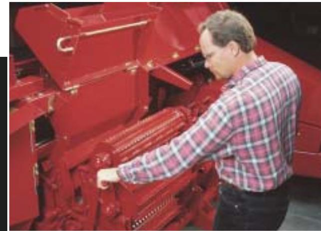
The Case IH feedrolls lift up for easy cleaning and inspection of the shearbar and smooth roll scraper. There's no need to take the feedrolls out of the machine, and no need to remove the crophead to lift the upper feedroll.
