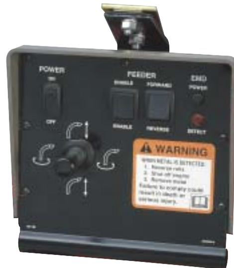
*A light and horn alert you when metal is detected. Just use the feedroll control switch to back the material out of the feedrolls. After the metal has been removed, the metal detector resets automatically.*
