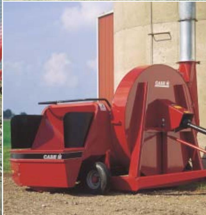
For a forage blower that can keep up with the FHX300 and your wagons and trucks, choose the Case IH 600 forage blower. It fills extra-tall silos fast to increase your productivity. Features include an auger-fed design and a 60-in. (1524 mm) diameter blower fan.
