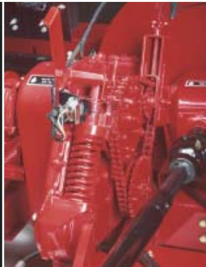
If you encounter extremely heavy material, an electric clutch allows you to control the reversing gearbox to easily unplug the head without leaving your tractor seat.
