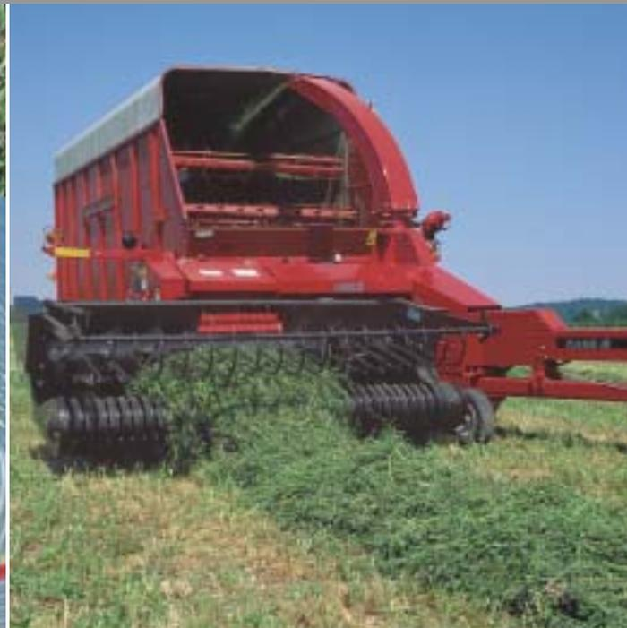
For high-capacity haylage production, choose the FHX300 with a 76.5- or 92-in. (1.94 or 2.34 m) tine-to-tine windrow pickup. Rows and rows of curved tines gently gather every bit of the windrow — even short or fine hay.
