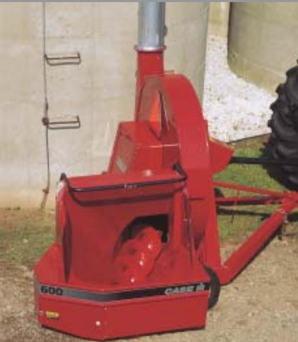
The 12-in. (305 mm) diameter auger is positioned at a 30° angle to the blower, providing smooth transitioning of material from the hopper to the blower. The high-speed auger breaks up crop slugs and eliminates plugging. A water inlet flange allows for proper water placement, which increases blower efficiency by removing the plant juices that gum up the blower and housing.
