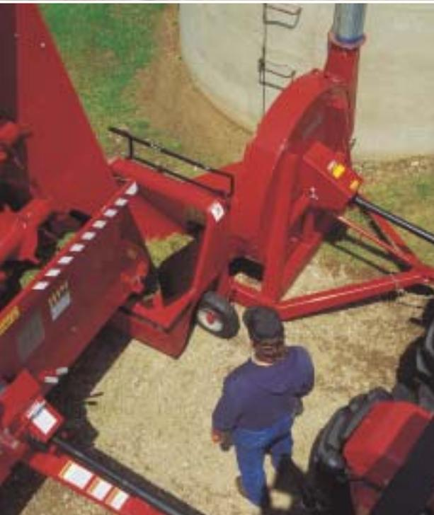
You can position wagons fast thanks to the wide 37-in. (940 mm) hopper that extends 20 in. (508 mm) past the blower housing. You'll have ample room for maneuvering into position and easy access to speed up your unloading time.
