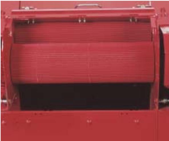
*The optional onboard crop processor is located behind the cutterhead. Chopped material passes directly to it from the cutterhead, minimizing the chance of plugging. For chopping haylage, the processor is easily bypassed by simply removing one baffle and the drive belt.*
