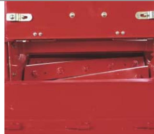
At the heart of the Case IH Model FHX300 is this 21-in.-diameter, 12-knife cutterhead. Hardened alloy knives span the full width of the cutterhead and chop evenly and efficiently, converting your crop into high-quality feed.
