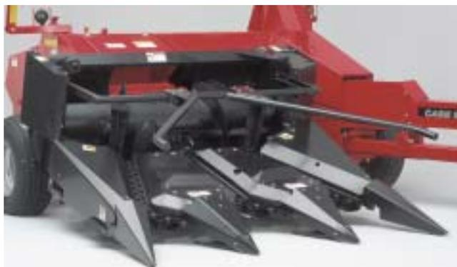
*The Case IH 3-row corn head grabs every stalk you grow, even in lodged crop conditions. The cutting discs shear corn close to the ground and are spring-loaded, allowing them to move out of the way when they encounter an obstacle.*
