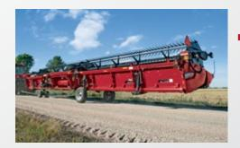
■ An industry-exclusive low-speed transport system (25 mph or less) allows the operator to deploy the transport package with the touch of a button, saving time when moving from field to field.
