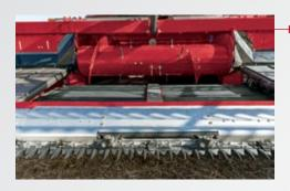
A seed saver channel along the bottom of the draper belt smoothly pulls grain into the combine, saving up to three percent more grain so no seed is left behind.
