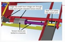
An upgraded suspension system features dual torsion blocks straddling the center knife drive, improving suspension in the header's center section and providing better flotation and improved range of rotation. Torsion blocks enable the operator to adequately adjust cutterbar pressure for even the most adverse conditions, such as soft fields and wet harvest conditions.
