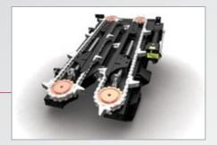
A large, open **front-gathering chain sprocket** sweeps stalks efficiently into rolls and helps harvest downed cornstalks.
