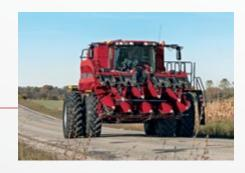
■ Case IH offers folding corn heads in 8-row and 12-row configurations. Capable of folding into transport mode in less than a minute, folding heads dramatically improving transport efficiency, and, ultimately, field productivity.
