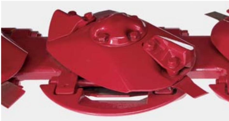
▲ **Independent disc modules** on the cutterbar make service and repair easy with bearings, gears and lubricant for each disc module individually sealed. Damage to one module does not spread to another. Ductile iron rock guards and easily accessible skid shoes will protect the cutterbed through many tough seasons.
