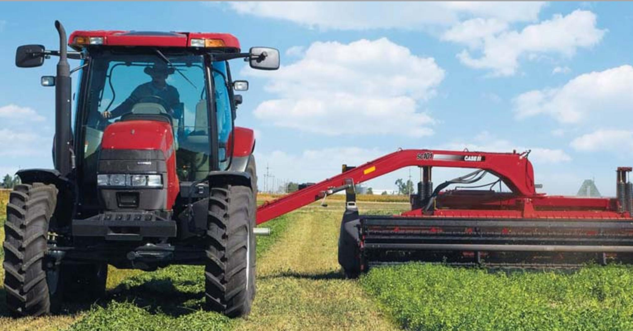
▲ Hydraulic header tilt allows up to 12 degrees of on-the-go adjustment to the cutting angle without requiring an additional hydraulic remote valve.
