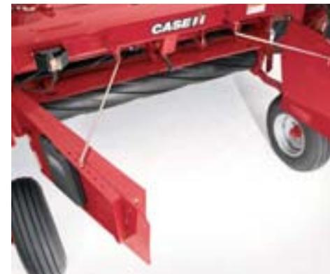
▲ No-tools adjustment of swathboard (above) and windrow shields (right) allow you to lay down a swath as wide as 8 ft. (2.4 m) or a windrow as narrow as 3 ft. (0.9 m). Shields fold flat for compact storage and less chance of shield damage.
