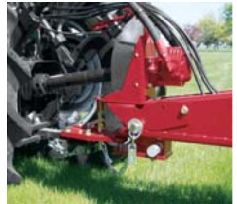
▲ Hydraulically driven, counter-stroking dual sickles provide smooth, clean cutting with less vibration and maintenance.
