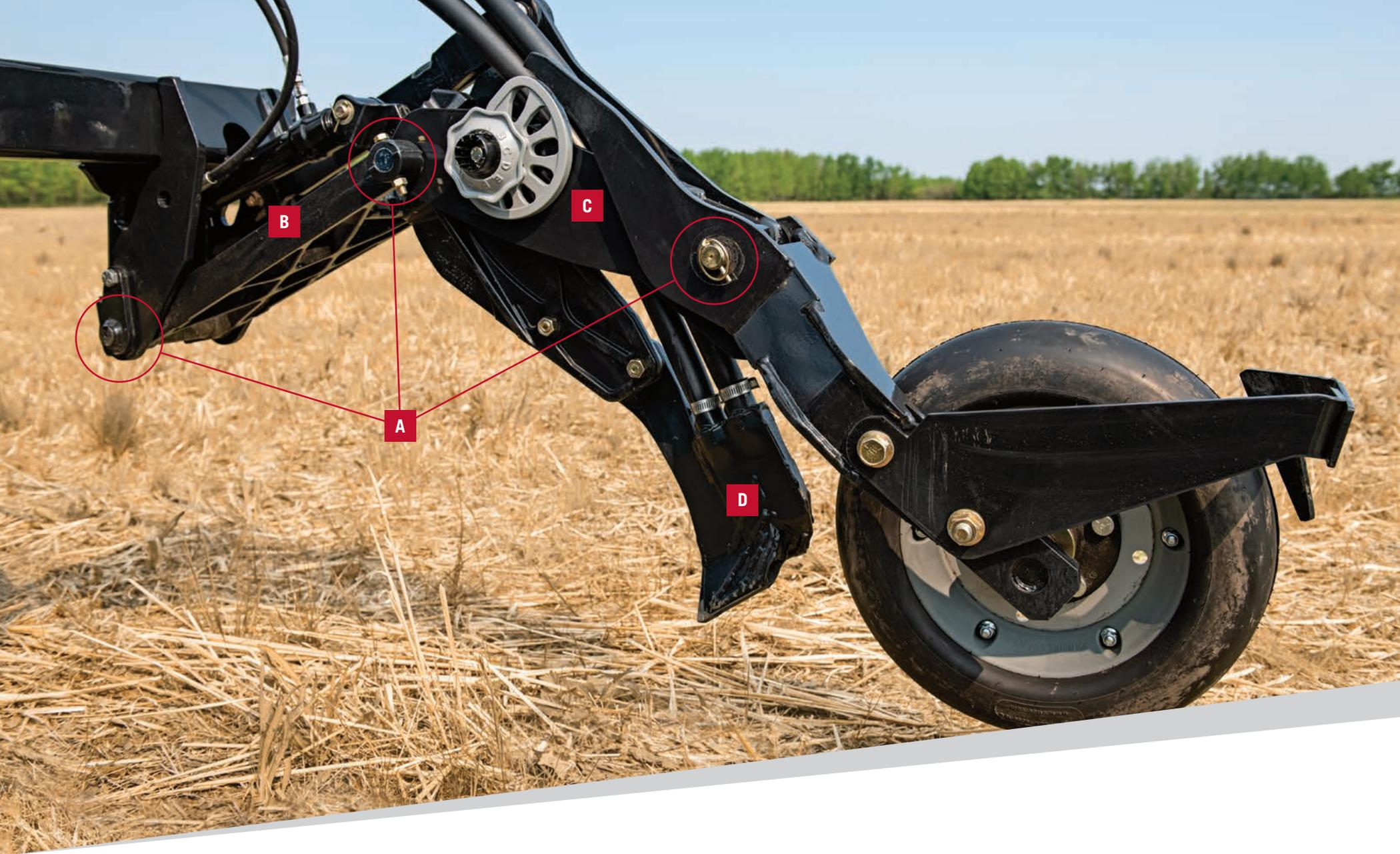
**A** Sintered metal bushings deliver maximum durability (multiple locations circled)
