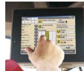
Folding operations, row unit-trip force, and down pressure adjustments are all at the operators fingertips and easily adjusted on the monitor.
