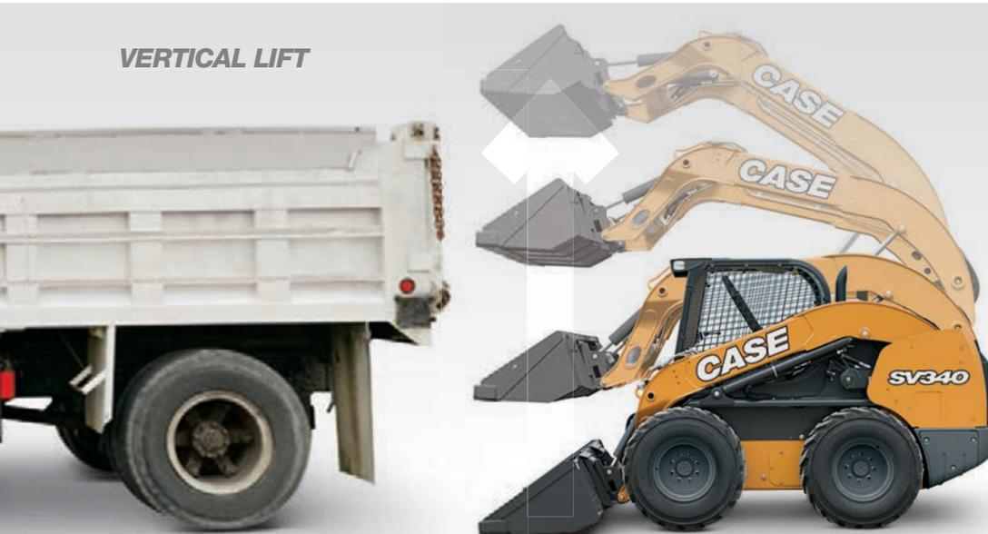
Vertical-lift machines are engineered for lift-and-carry and truck-loading jobs. The geometry of the dual arm allows the load to rise directly up, providing maximum reach at full height. Vertical-lift machines are ideal for reaching over the side of and into the middle of high-side trucks.
