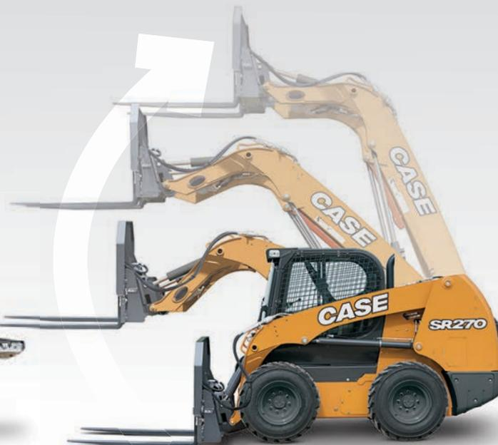
Radial-lift machines are engineered for digging, prying and pushing. The angle of the arm ties directly into the chassis for superior strength when digging and pushing. It also provides maximum reach at the operator's head height, making it perfect for loading and unloading pallets from trucks.
