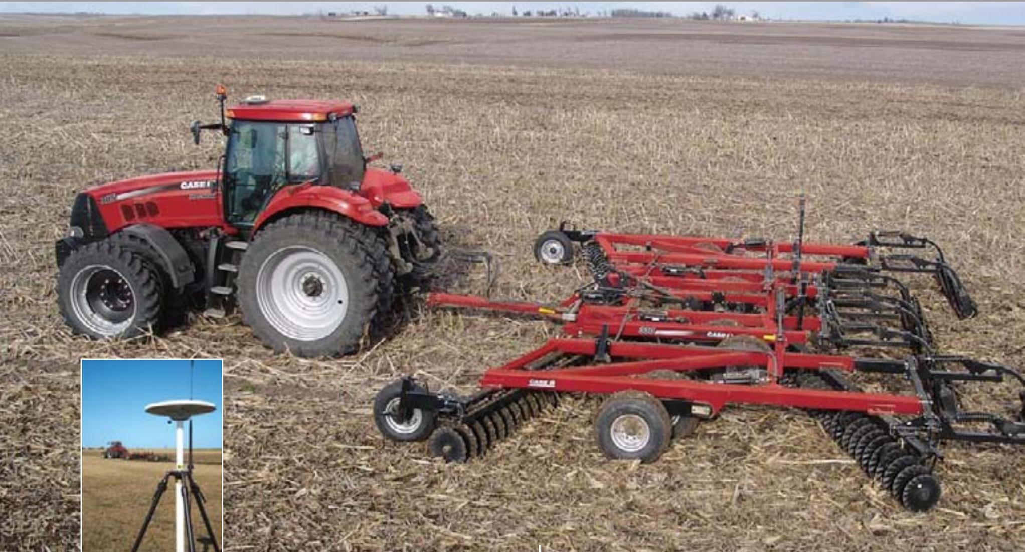
▲ Driven with an **AFS ACCUGUIDE™** autoguidance system at 7.5 to 9 mph (12-14.5 kph), the Turbo 330 can cover ground more quickly – up to 25 acres per hour with the 25-ft. (7.6 m) machine, and up to 35 acres per hour with the 34 ft. (10.4 m) machine.
