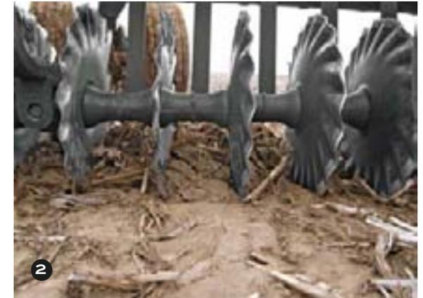
Removes surface compaction and crusts.
