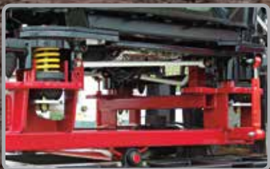
Steiger 4-point cab suspension - the first in the industry - shown here.
