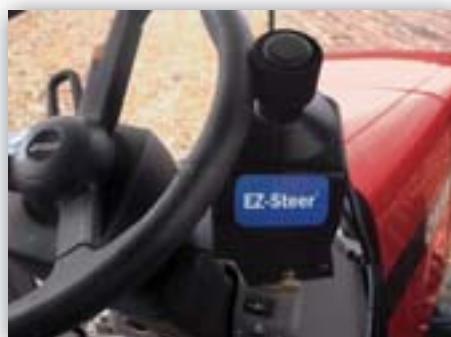
The EZ-Guide 500 will control the EZ-Steer assisted steering system.
