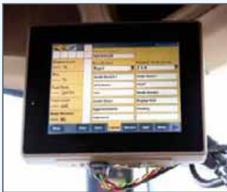
Use the new Case IH AFS Pro 600 display to control AFS AccuGuide autoguidance systems, 1200 Series planters, and Axial-Flow combine yield monitoring and mapping systems.
