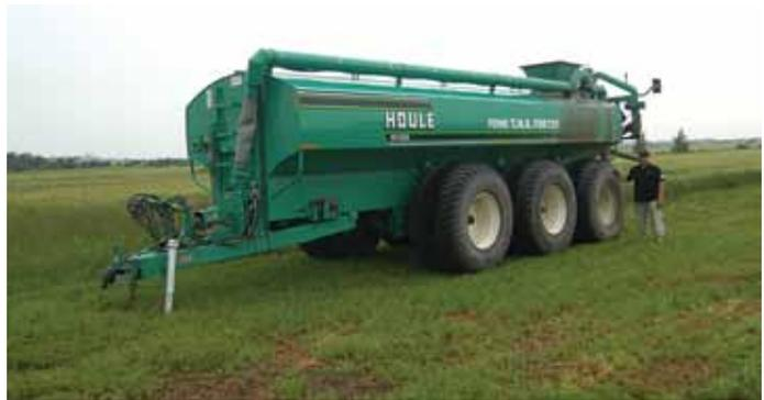
**The Fortins pull this 6,000-gallon liquid manure tanker on 6- to 12-mile (10- to 20-kilometer) round trips with the Puma 225 CVT. Loaded, the tanker weighs around 60,000 pounds (27,215 kilograms) and has its own hydraulic brakes. They say the CVT is a good match for managing the load.**
