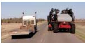
**The Precision Hoe 800 air hoe folds to 17 feet 8 inches wide for transport.**
