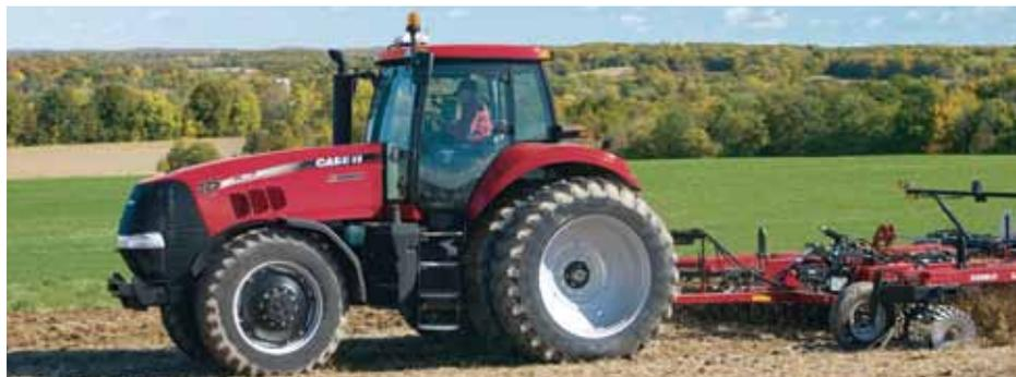
The new Magnum 180, 190, 210, and 225 tractors share the Surveyor cab and frame with the higher-horsepower Magnum models. Efficient new CVT transmissions are available on all these new Magnum models.
