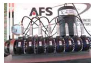
**Air-activated clutches manage row units to eliminate planter overlap.**
