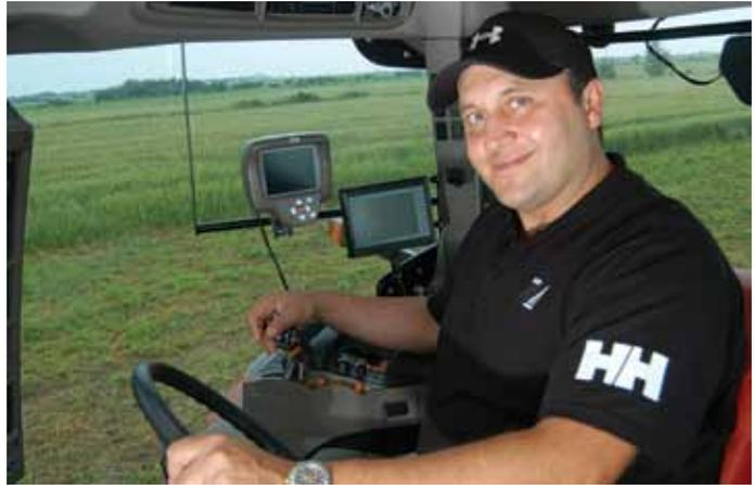
**Stephane uses the tractor's Multicontroller lever to select ground speed; the tractor's AutoProductivity Management system automatically chooses the most efficient combination of engine rpm and transmission ratio to handle the load.**
