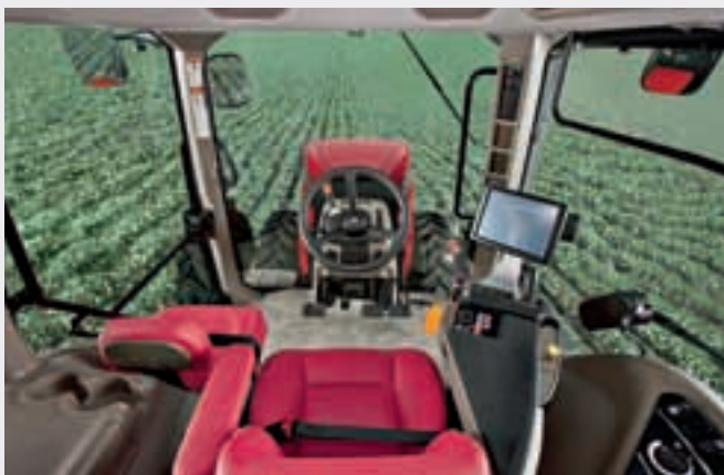
Magnum and Steiger cabs have new features to enhance comfort and productivity. A new MultiControl Armrest puts six key functions at your fingertips. The new AFS Pro 700 color display is integrated into the armrest, and features a large touchscreen with a smaller overall profile for increased visibility.
