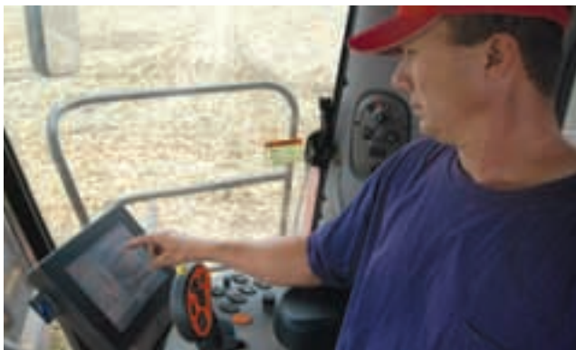
Tim Martin is in his second year of making site-specific yield maps, with the goal of maximizing the economic yield of each field. The Martins' AFS AccuGuide autoguidance system with RTK accuracy is a good match for their strip-till planting and drip irrigation systems.
