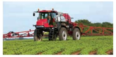
them to the previous height using a single switch; AFS AccuGuide autoguidance; AIM Command pulse width modulation to manage droplet size for consistent accurate application under varying conditions; AccuBoom automatic boom section control; high-intensity discharge (HID) lighting; and the AFS Pro 700 color display for a single interface for sprayer control and autoguidance.
