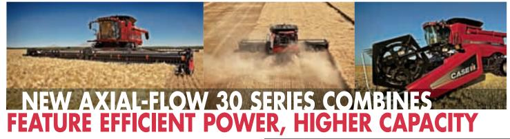
The latest model series of Case IH Axial-Flow combines use selective catalytic reduction (SCR) technology to meet Tier 4A emissions requirements, with higher horsepower and improved fuel efficiency.
