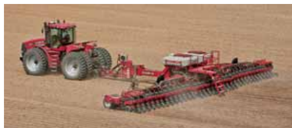
The 1260 Early Riser front-fold planter is available in 32-row 30-inch (76.2-cm) models and 36-row models with 20-, 22-, or 30-inch (50.8-, 55.9-, or 76.2-cm) row spacings.
