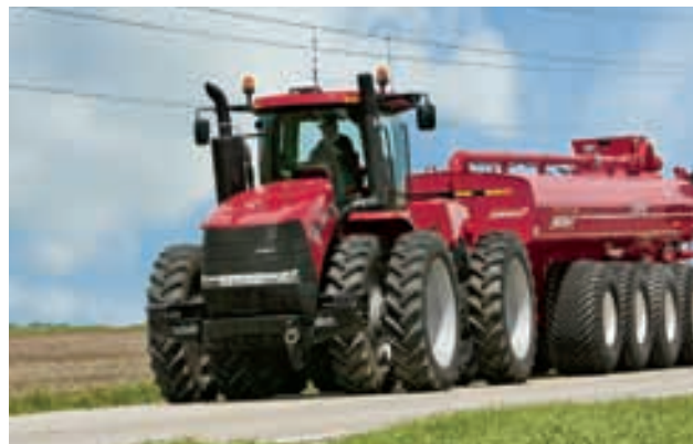
Optional engine brakes and trailer brakes for Steiger and Magnum tractors provide added control for transporting heavy loads.
