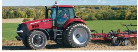
The new Magnum180, 190, 210, and 225 tractors share the Surveyor cab and frame with the higher-horsepower Magnum models. Efficient new CVT transmissions are available on all these new Magnum models.
