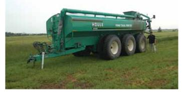
The Fortins pull this 6,000-gallon liquid manure tanker on 6- to 12-mile (10- to 20-kilometer) round trips with the Puma 225 CVT. Loaded, the tanker weighs around 60,000 pounds (27,215 kilograms) and has its own hydraulic brakes. They say the CVT is a good match for managing the load.
