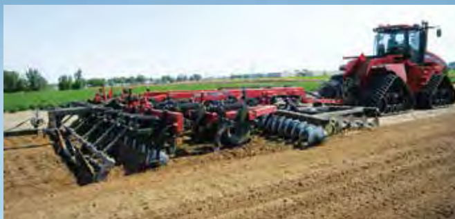
Dave Sparks uses a 26-foot Case IH Ecolo-Tiger 870 pulled by a Quadtrac 600 tractor in his custom tillage business. He goes into high-residue irrigated fields and leaves them smooth, deep-tilled and ready to plant after two passes.
