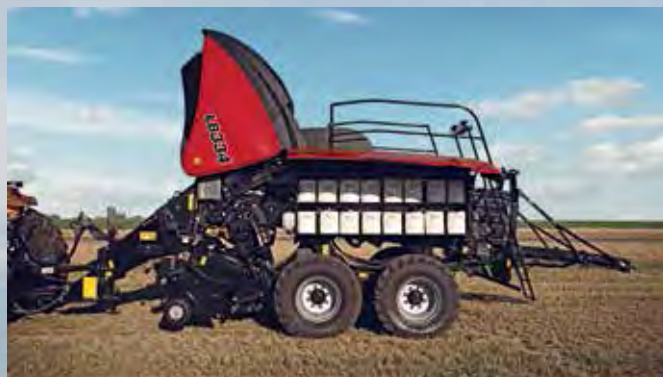
The large easy-opening hood and side panels provide access to all service points. Up to 16 twine balls can be carried on each side.
