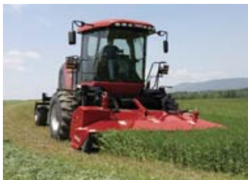
Match the 13-foot RDX131 rotary disc header to WDX1902 or WDX2302 windrowers.
