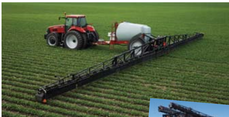
New pull-type sprayers include the SRX100 with a 1,000-gallon tank (shown) and the SRX160 with a 1,600-gallon tank. Forward-folding spray booms are offered in widths from 80 to 134 feet.
