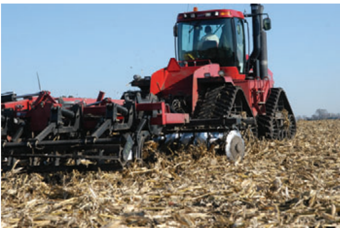
In these conditions, the Quadtrac 535 tractor pulled the 22-foot 11-shank Ecolo-Tiger 870 steadily at about 5.5 mph. The Ecolo-Tiger is designed to perform effectively in the 5- to 7-mph range.
