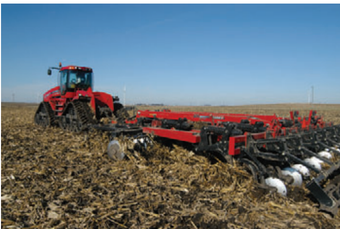
In the heavy black damp soils, the Ecolo-Tiger 870 mixed residues with soil, opened the soil for air and water to penetrate, broke a compaction layer, and leveled the surface. A prior pass with a Case IH True-Tandem 330 Turbo helped size the residues from the 200-bushel corn.
