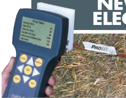
The ProID system generates an RFID tag containing production information for each bale.
