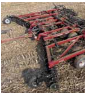
Twenty-inch diameter shallow concavity turbo vane blades on 7 1/2-inch spacings run at just 1 1/2 to 2 inches deep to lift, size and mix soil and residues.
