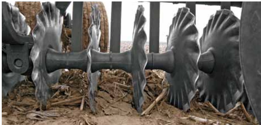
Twenty-inch diameter shallow concavity turbo vane blades on 7 1/2-inch spacings run at just 1 1/2 to 2 inches deep to lift, size and mix soil and residues.
