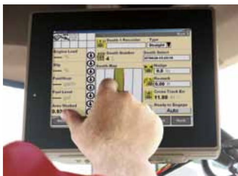
The Case IH AFS AccuGuide All-Makes autoguidance system lets you use the full-featured Case IH AFS Pro 600 monitor for autoguidance on legacy Case IH Magnum and Steiger tractor models and to control Case IH 1200 Series planter and air drills.
