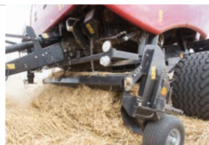
The five-bar pickup collects even very short crop reliably at high driving speeds.
