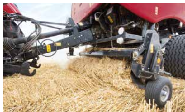
The five-row pickup reliably collects even very short crops at high speeds.
