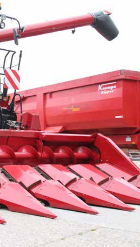
Rainer Uckelmann (top left) has now set himself in business independently with the service of corn stubble harvesting. The combine harvester is equipped with a front-mounted corn picker attachment arranged behind the folded up stubble bunker.
