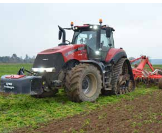
The Magnum Rowtrac breaks up parsley root mass prior to ploughing, using a Pottinger disc/ tine cultivator
