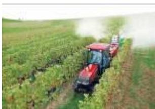
The four Case IH Quantum V models from 78hp to 106hp share a similar mechanical configuration to Quantum F tractors, but with a maximum cab height of 2190mm and a minimum width of just 1190mm.
