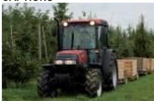
Case IH Quantum F models from 88hp to 106hp are designed for use on fruit farms and other applications which require high power output, compact dimensions, narrow width and a tight turning radius.
