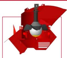
New 4 blades extractor cleaning system - The Case IH exclusive Antivortex system reduces vegetable impurities and cane loss and increases load density. With it, the power demanded by the extractor has been reduced compared to a conventional system, reducing vibrations and fuel consumption.
