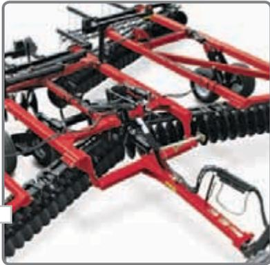
The Pull Frame features an increased section of pull plates and 9.5 mm (375 in.) wall tubing for added durability.
