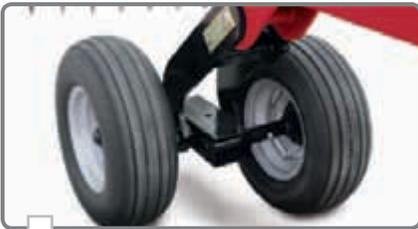
Walking tandems on mainframe and wings offer more consistent depth control, better handling in wet or soft soil and a smoother ride leading to less stress on the frame.
