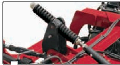
The heavier springs provide solid stability for transport and minimize “rocking.” There is no need to re-level the machine when changing from field use to transport position.
