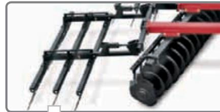
Rigid Arm Scrapers work best in heavy soil, low residue conditions, while Flex Arm Scrapers work in lighter soil or high residue conditions to keep blades free of mud and residue.
