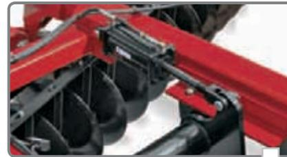
The rockshaft, clamps and angle mounts provide great strength for the weight and size of the True-Tandem 370 disk.
