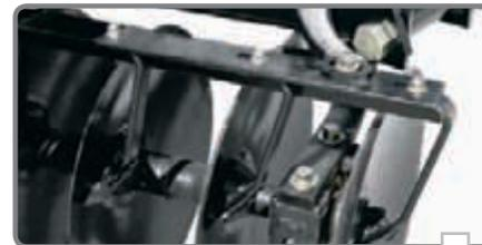
For uniform residue and soil mixing, even in the center between disk gangs, Case IH offers a center shank to remove the uncut soil between disk gangs. The center shank is located farther from the front blades than prior models and has increased holding force.
