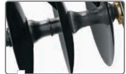
Earth Metal® blades feature a crimped-center design for increased blade strength and shallower concavity for better soil penetration with minimized soil compaction. The blades are mounted on nodular cast iron spools for even greater strength and durability.
