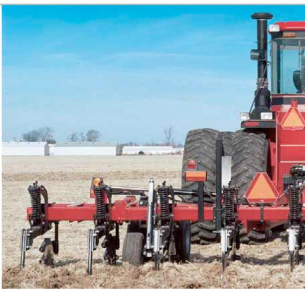
▲ Parabolic Shanks w/7-inch tiger® points and 6-inch Coverboards – the most aggressive tillage option.
