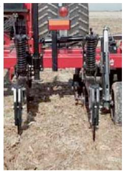
No-till shanks and 8-inch No-till points provide excellent fracture of compaction to increase water absorption and air exchange. When combined with Case IH berm tuck'r row sealers, this tillage system provides disturbance-free tillage - a very effective system for No-till or HEL ground.
