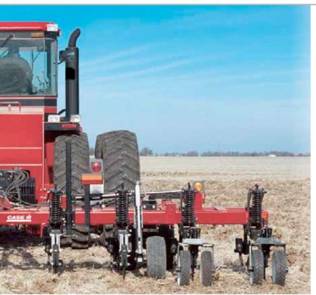
▲ No-till Shanks and 8-inch No-till Points – even less soil disturbance than the MRD shank.
