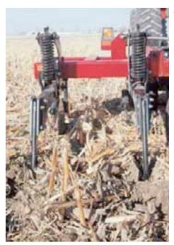
■ Parabolic shanks with optional 7-inch tiger points and 6-inch coverboards are the most aggressive tillage option. The parabolic shank is a 1-1/4 x 3-inch edge-bent shank that lifts and fractures compaction and covers more residue than straight shank designs.
