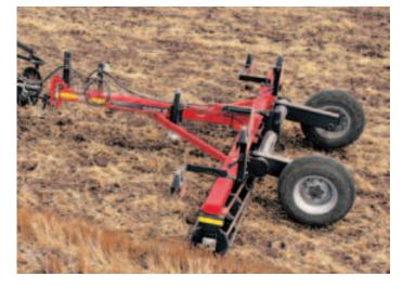
5 cm straight points Used for prefracturing on lead shanks.
