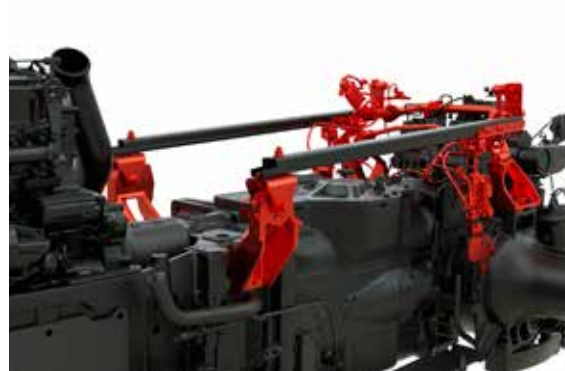
The semi-active, hydraulic cab suspension reliably absorbs jolting and vibrations.
