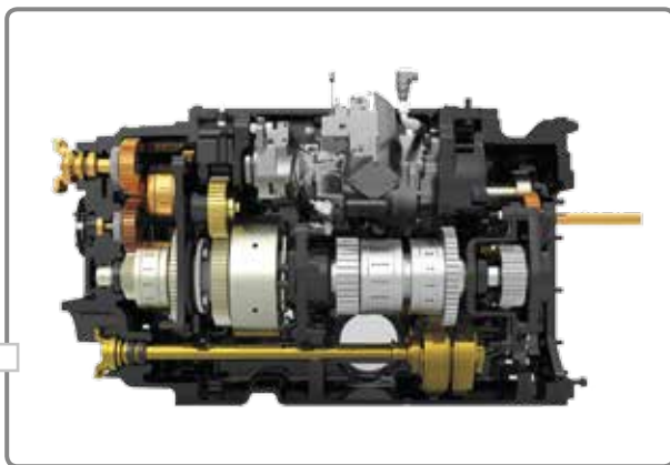
CVT transmission – stepless drive between 0-50 kph.
