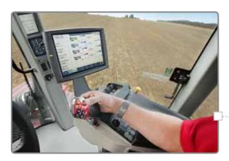
The operation of the control valves are easy handled through .......... the Joystick and is standard on tractors ordered with 8 valves.
