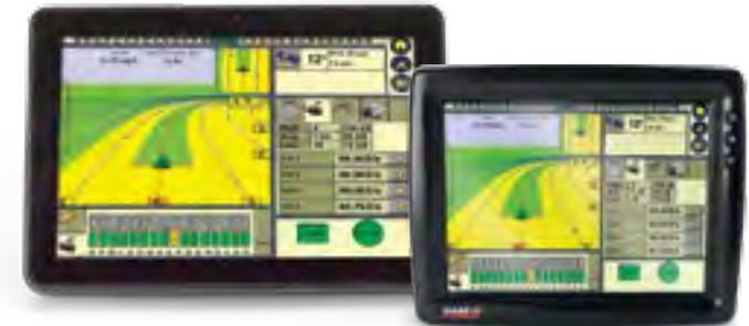
The XCN-2050 and FM-1000 displays in the tractor communicate guidance information to the TrueTracker system, providing repeatable accuracy to improve seedbed and nutrient placement, helping to enhance crop stands and yields.
