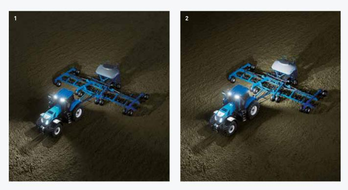
Two cab LED lighting packages are available, including Level 1 with 18 lights (photo 1), and Level 2 with 24 lights (photo 2). Both come in various configurations to suit your individual requirements.
