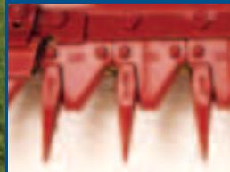
Bolt-on, over-serrated, back-hardened knife sections with adjustable hold-downs are standard equipment.
