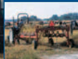
The HT152 standard and HT154 deluxe wheel rakes both fold down to a narrow 8' 3" for easy transport. The hydraulic-fold frame lets you do it right from your tractor seat.
