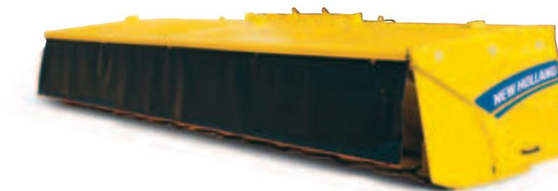
Delivering one-pass, high speed harvesting, the six metre Marangon for New Holland header scythes through whole crop and grass thanks to its 14 cutting discs which guarantee a super fine cut.
