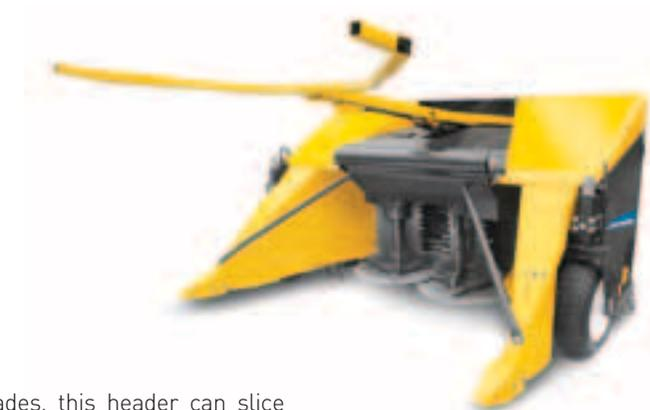
Featuring two saw blades, this header can slice through stems of up to 150mm making it the default choice for energy growers.
