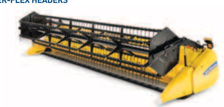
Maintain uniform stubble height in uneven fields. How? The header flexes up to 10cm to follow the ground contours perfectly thanks to an exclusive and patented rubber spring floatation system.
