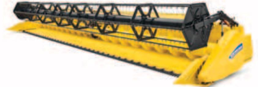
Varifeed™ headers benefit from a full 575mm of knife adjustment for guaranteed harvesting efficiency and correct feeding. What's more, you can adjust the knife position right from the comfort of the cab.
