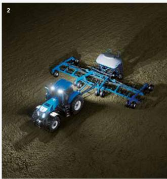
Two cab LED lighting packages are available, including Level 1 with 18 lights (photo 1), and Level 2 with 24 lights (photo 2). Both come in various configurations to suit your individual requirements.
