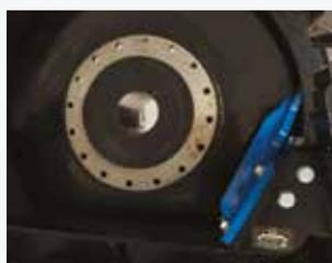
A heavy-duty scraper cleans the drive wheel and drive lug area of dirt and debris to avoid misalignment and increased belt wear.
