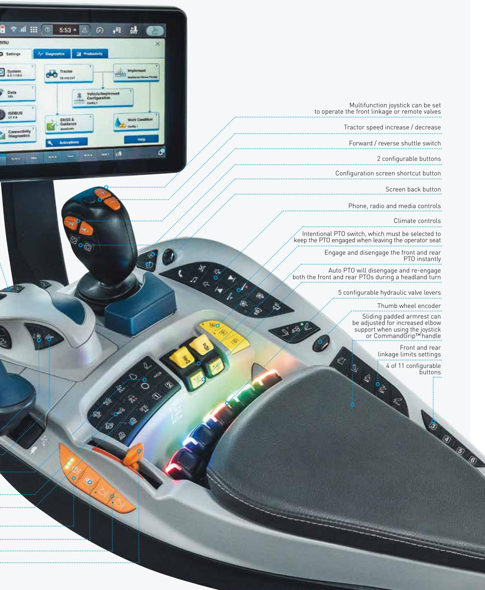
Multifunction joystick can be set to operate the front linkage or remote valves
