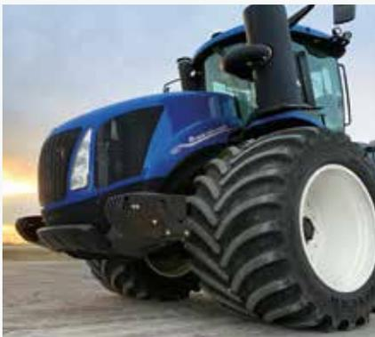
When equipped with LSW1250/35R46 singles, the overall width measures about 150 inches or 12.5 feet. This narrow roading width, in combination with a light footprint, provides a middle ground when choosing between SmartTrax and high-flotation duals.
