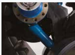
An integrated accumulator/tensioner automatically adjusts belts for proper tension.
