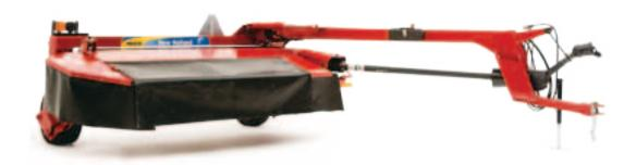
Tractor hook-up is easy. Simply drop in the pin, hook up the PTO and three hydraulic hoses. The primary PTO uses an 80-degree constant velocity joint that permits tight turning. If desired, your dealer can order an optional secondary PTO assembly with CV joint that allows you to steer the machine around field obstructions on-the-fly.
