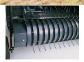
**OPTIMUM CROP TRANSFER** The long pick-up tine guards and two short side augers ensure a smooth, uninterrupted crop flow to the feeder.
