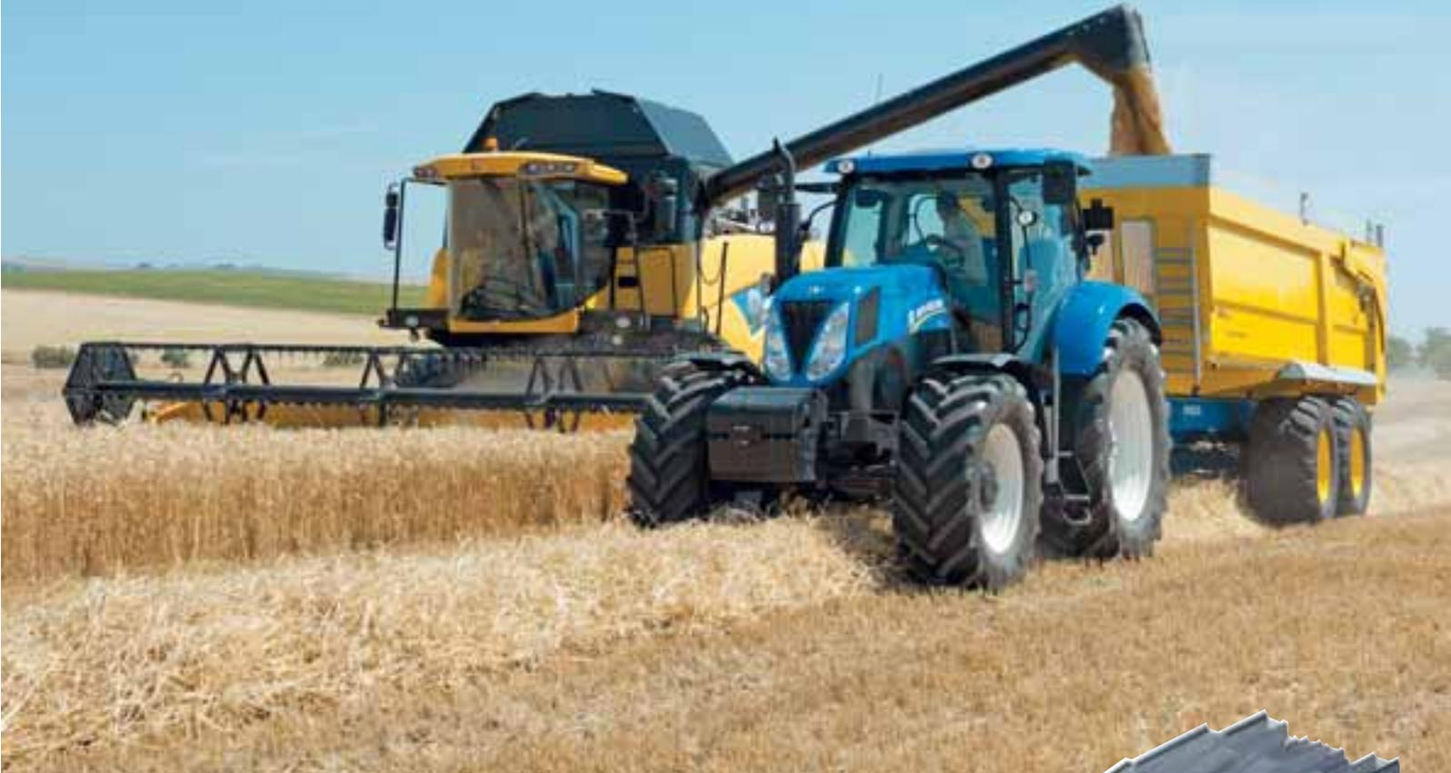
New Holland CX5000 and CX6000 combine models benefit from the four-drum technology: threshing drum with Opti-Thresh™ system, beater, Rotary Separator, and Straw Flow™ beater. Extremely versatile, the system can be adapted to suit a wide variety of crops and different harvesting conditions with no compromise in kernel and straw quality or throughput.
